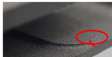
Fig (3) NC produced applying fillet to the radius on the tangent point.
